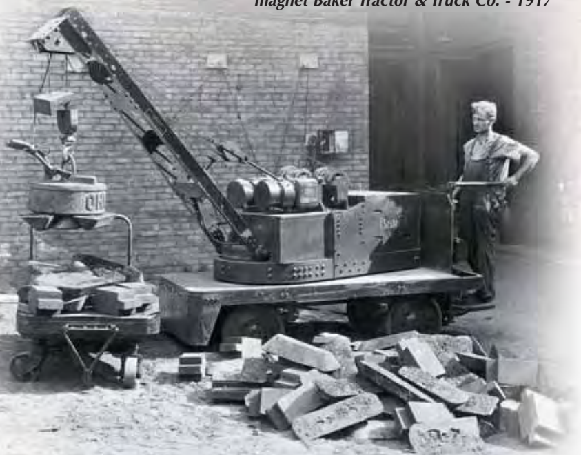
Lifting pig iron ingots with 20" Ohio Magnetics magnet Baker Tractor & Truck Co. - 1917
